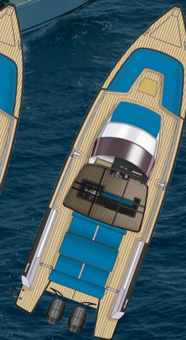
main deck option with galley and aft bench with lowerable cockpit table
